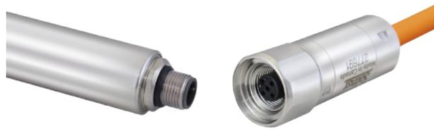
Line up the alignment pin on the AquaVent logger connector with the alignment socket in the Vented Cable connector. **Once properly aligned**, carefully push the connectors together.
