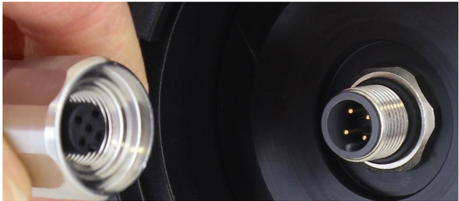
Once properly aligned, carefully push the connectors together, using your thumbs as guides.
