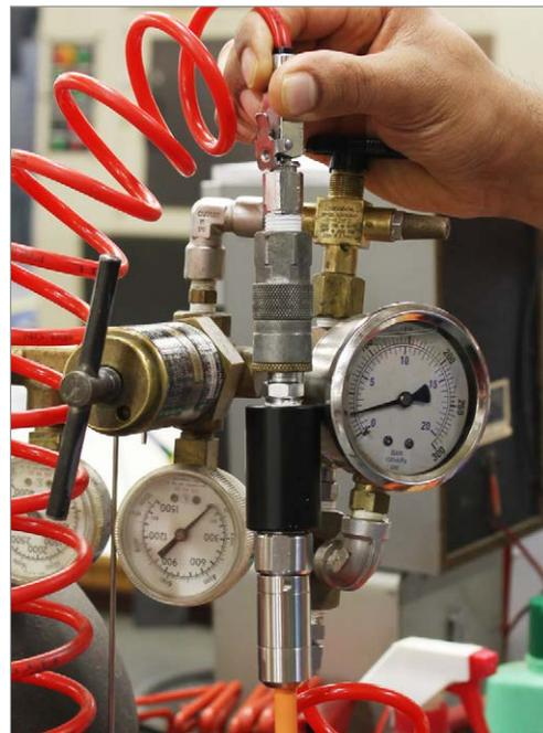
Figure 9-6 Nitrogen Gas Being Blown Through the Vented Cable
