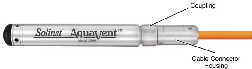
Twist the stainless steel coupling while holding the stainless steel cable connector housing still. Twist the stainless steel coupling until it seats. **Do not twist the Vented Cable or the logger.**
