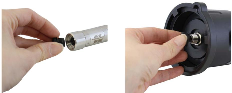
Remove the storage caps from the connectors on the Wellhead and Vented Cable.
