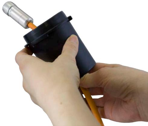
Bring the Vented Cable through the bottom of the well cap sleeve.
